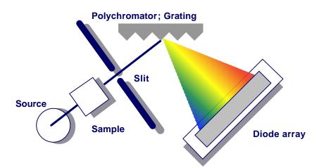
Figure 1. Schematic of photodiode array spectrophotometer
