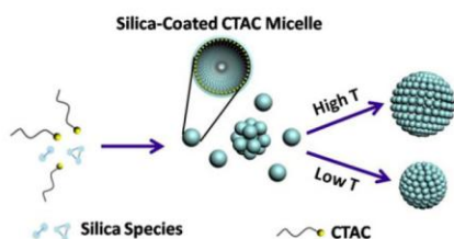
Scheme 1. The formation process of MMSNs through spherical micelle templating mechanism. (1) silica-coated CTAC micelles are formed through the co-organization of silica precursors and surfactant CTAC; (2) aggregation of a part of silica-surfactant composite micelles into disordered spherical nanospheres; (3) the primary-generated small particles grow homogeneously into bigger particles, and finally form monodisperse mesoporous silica nanospheres (MMSNs). The size of MMSNs increases as the reaction temperature increase.
