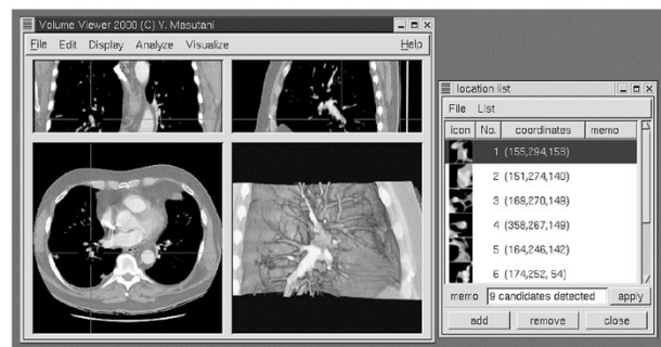
Fig. 10. Display system for detection result. By pointing a candidate on the right list, three sectional views of axial, coronal, and sagittal planes are displayed.
