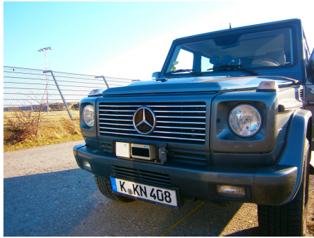
Fig. 2. SICK LD-MRS laser scanner mounted on the SOL-Car
