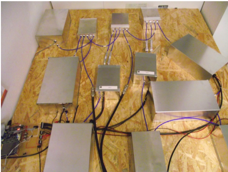
Fig. 4. Physical topology of Ko-TAG emulator (current functional prototype status)
