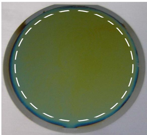
**Figure 2.** (Color online) Electrochemically etched (100) p-type Ge wafer, 50 wt % HF,  $j = 1 \text{ mA/cm}^2$ , and  $t = 3 \text{ h}$ . Note that the dashed line represents the region at which the porous layer thickness has a maximum variation of 30 nm.
