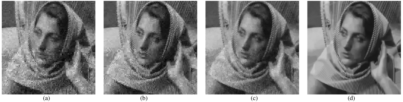
Fig. 10. CS recovered image Barbara (25% measurements). (a) TSW (21.82 dB, FSIM = 0.7481). (b) TSDCT (23.65 dB, FSIM = 0.8231). (c) TV (25.18 dB, FSIM = 0.8403). (d) RCoS (29.60 dB, FSIM = 0.9123).
