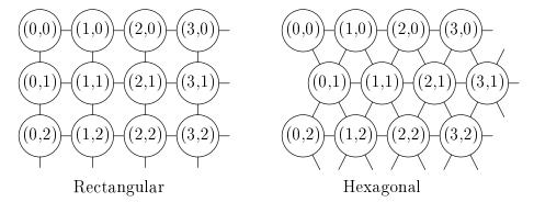
In the picture above the locations of the units in the two possible topological structures are shown. The distance between two units in the map is computed as an Euclidean distance in the (two dimensional) map topology.
