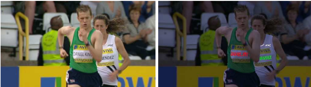
Figure 5: OCR results for candidate text lines. The red line is read as “DANIEL KIN” with OCR confidence 83, the white one as “MMM” with OCR confidence 15, and the green one “IENDEZ” with OCR confidence 69. The OCR confidences here act as a filter on the candidate athletes’ names.
