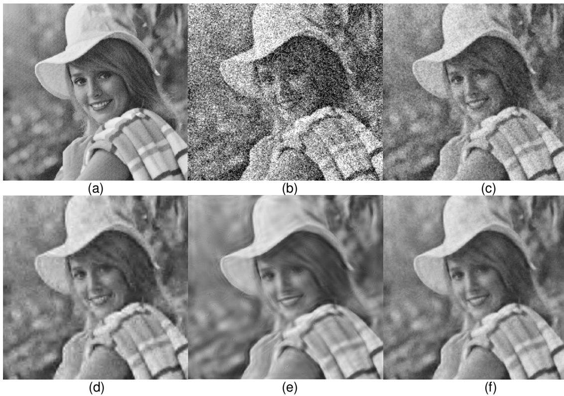
FIGURE 3: GIRL test image: (a) Original image, (b) Noisy image with \sigma = 50 dB, (c) Image after denoising with Gaussian filter, (d) Denoised image from BayesShrink Wavelet Thresholding, (e) Denoised image from Curvelet transform, (f) Denoised image from Proposed method.
