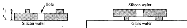
Fig. 2(a) Processed silicon wafer (upright) (b) bonding of silicon wafer (inverted) to glass
