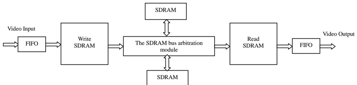
Figure 4. Pong operation procedures schematic.
