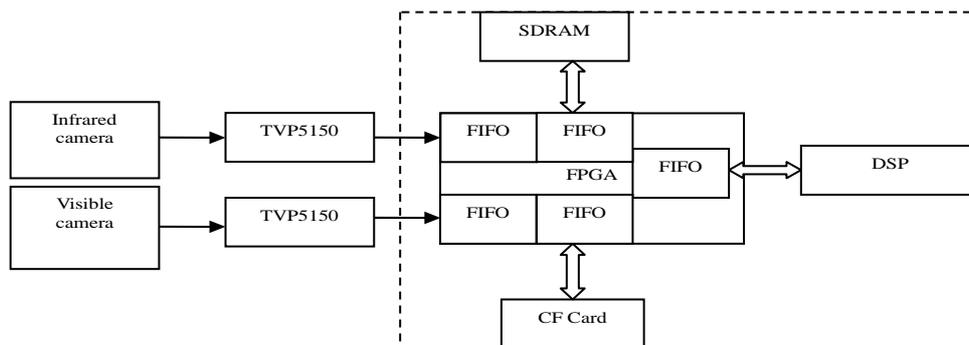
**Figure 2. The structure diagram of video data acquisition and storage.**
