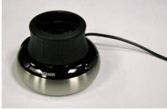
Figure 4.2: The 3DConnexion brand SpaceNavigator USB controller. The knob, designed for navigating through 3D environments, can be moved laterally from left to right and front to back, pushed and pulled vertically, tilted from side to side and from front to back, and twisted around its center axis, yielding six features describing its position.
