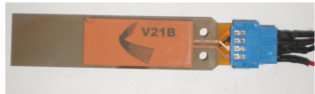
(a) Piezoelectric Harvester
