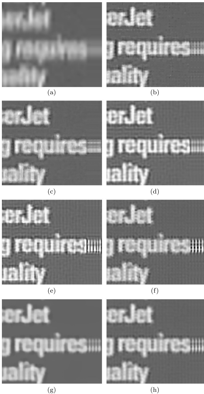
Fig. 7. HR images obtained from the first 20 LR frames of the text sequence using: (a) BBC, (b) RSR, (c) ZMT, (d) SAR, (e) TV, (f) \ell_1 , (g) TV-SAR with \lambda_3 = 0.8 and (h) \ell_1 -SAR with \lambda_2 = 0.4 .
