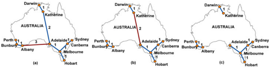
Fig. 1. (a) The MST_p created from 10 Australian cities (actual locations of the cities in the map are schematic). The edge between “Albany” and “Adelaide” is the candidate for deletion as the neighborhood value p > \lfloor \ln(10) \rfloor = 2 (b) In the first iteration of MST_{kNN}^+ the edge between “Katherine” and “Adelaide” is the next candidate to delete as p > \lfloor \ln(7) \rfloor = 1 , where the number of elements in that component is 7 (c) Final clustering result.
