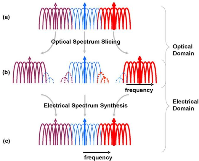
Fig. 2. Optical-to-electrical conversion of three OFDM bands via optical spectrum slicing and electrical spectrum synthesis. (a) The three OFDM bands in the optical domain; (b) OFDM bands after gapless optical spectrum slicing; (c) The three OFDM bands in the electrical domain after electrical spectrum synthesis. The arrows stand for the position of the comb lines. The dashed spectral components are eliminated through electrical spectrum synthesis.
