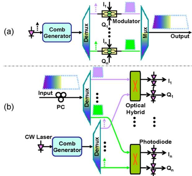
Fig. 1. (a) Transmitter and (b) receiver of Tb/s coherent optical OFDM systems using optical frequency combs. Dashed arrows and boxes illustrate the optical spectra at various stages. PC: polarization controller.
