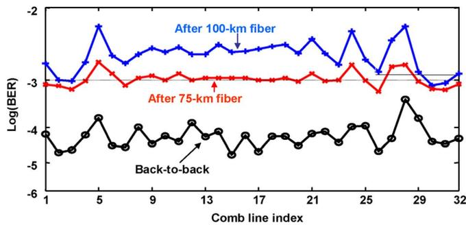
Fig. 6. BER of individual OFDM bands before and after 75-km and 100-km fiber transmission, respectively.
