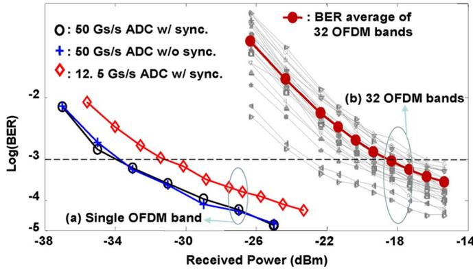
Fig. 5. Optical back-to-back BER measurements for (a) single OFDM band, (b) 32 OFDM bands. The gray and thin curves are the BER of individual OFDM bands.
