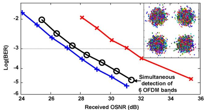
Fig. 10. Optical back-to-back BER measurements with the silica PLC. The two curves with crosses are the results of individual measurement of two OFDM bands. The curve with circles and the inset constellation are the results of simultaneous detection of six transmitted OFDM bands in two received optical spectral slices.
