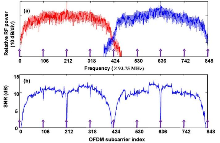
Fig. 8. (a) Received RF spectra of two optical spectral slices. (b) SNR estimation for all the OFDM subcarriers in the received two bands. The arrows on the horizontal-axes indicate the transmitter comb line position.
