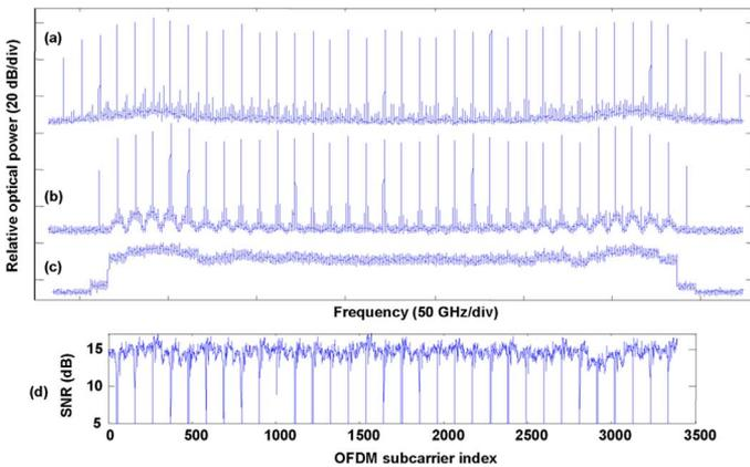
Fig. 4. High-resolution optical spectra of (a) after the comb generator, (b) after the DI filter and the bandpass filter with sharp edges, and (c) the generated 1.008-Tb/s optical OFDM signal. The spectra's vertical-axes are shifted for display and they are measured by the swept coherent heterodyne method with a resolution of 100 MHz. (d) The estimated electrical SNR performance for all of the OFDM subcarriers. The comb lines in (a) and (b) are aligned with the SNR dips in (d).
