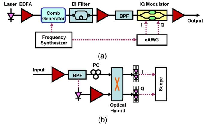
Fig. 3. (a) Transmitter and (b) receiver setup of Tb/s coherent optical OFDM. DI: delay interferometer; PC: polarization controller; BPF: bandpass filter; eAWG: electrical arbitrary waveform generator. EDFA: erbium-doped fiber amplifier. Dashed lines are electrical connections.
