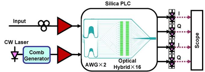
Fig. 7. Receiver setup using a silica PLC (with the layout design) for the detection of two optical slices. The PLC outputs multiple spectral slices but only two are used. AWG: arrayed-waveguide gratings.
