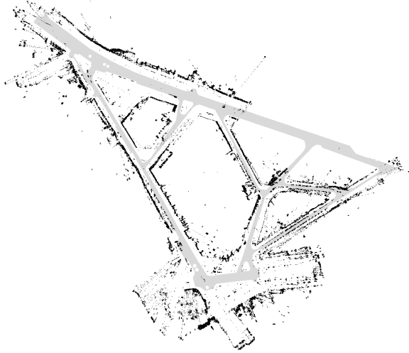
Fig. 7. Result of an accumulation mapping, black refers to occupied cells, gray refers to the road space provided by IGN
