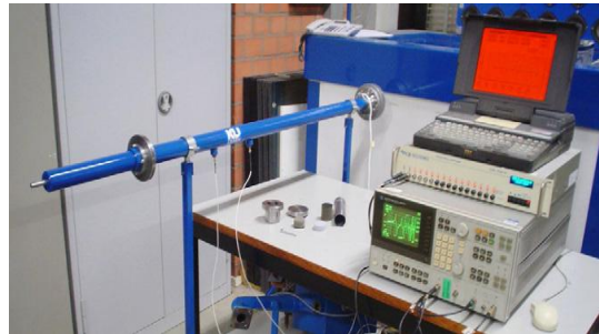
Figure 9: Laboratory setup for acoustic impedance measurement
