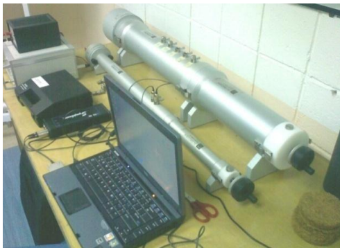
Figure 8: Experimental set up for experiment in impedance tube.
