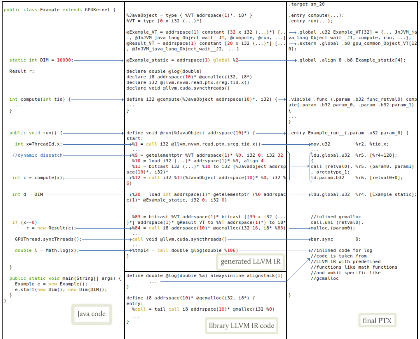
Figure 5: The flow of code transformations
