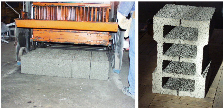
Fig. 12. Production of precast concrete blocs from masonry lightweight aggregates.
