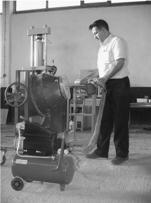
Fig. 1. Water spraying into mixer.
