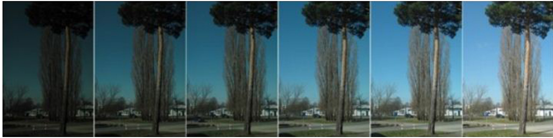
Fig. 2. Sequential color switching of a thermochromic laminated glass [4].
