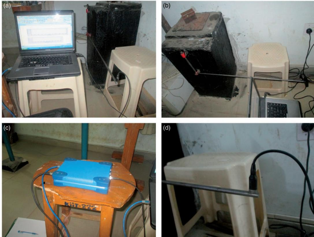
**Figure 14.** (a) Vibration indicator (NVgate Environment software); (b) cantilever shaft with frame; (c) vibration analyzer; (d) vibration pick-up with shaft.
