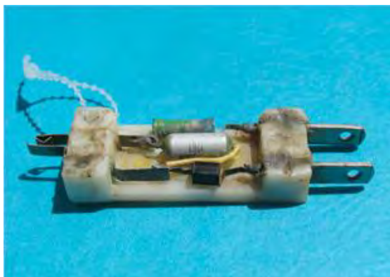
Figure 3. Battery Charger for battery non-rechargeable (two capacitor, one diode), 2007. Source: © Ernesto Oroza
