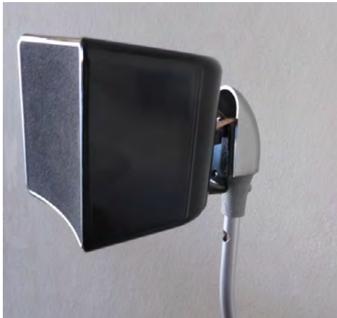
Figure 5. Replacement loudspeaker bracket. Source: Oya Demirbilek.
