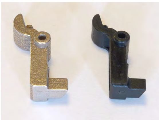
Figure 4. Panasonic SD257 bread maker original and improved latch. Source: Susan Parker.
