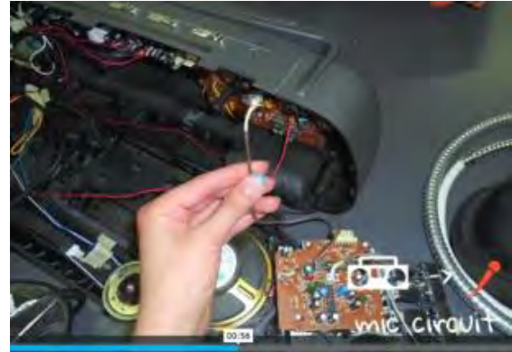
Figure 10. Students hacking the circuit to include a microphone (the shower components) and to connect a mp3 player.
