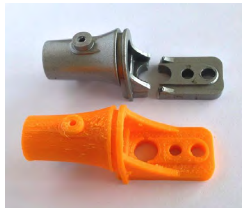
Figure 4. Original part showing failure and improved design. Source: Author
