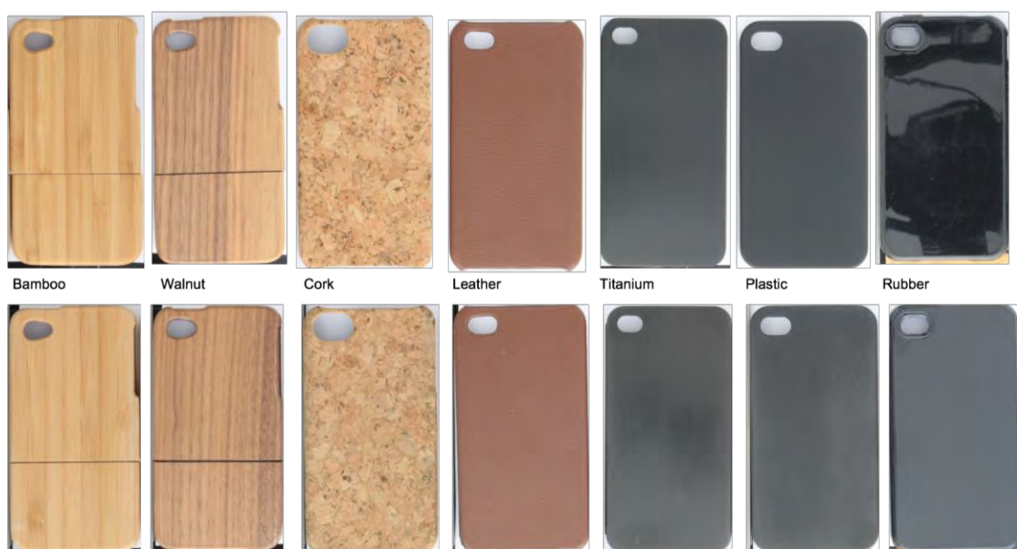
Figure 1. Mobile phone cases used in the study. New (top) and after gentle artificial ageing (bottom). Despite careful use of diffuse lighting the shiny new rubber (top right) shows reflections.
