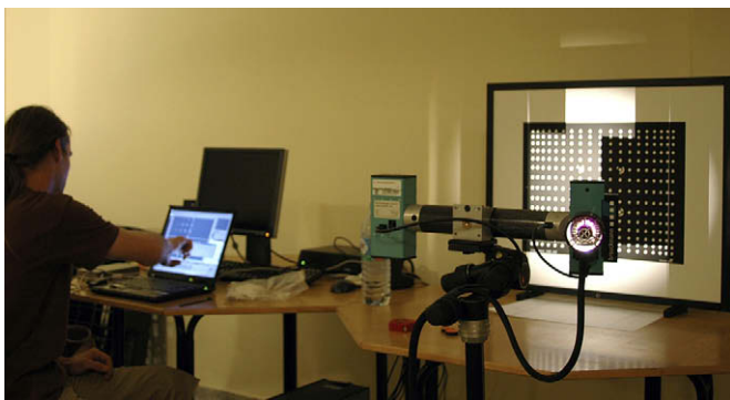
Fig. 5. Calibrating the scanner. The scanner is in the foreground on the right. It is projecting a structured light pattern on the calibration plate which is set at a fixed distance and angle from the instrument (note paper guide under the calibration plate). The calibration process is controlled by the software running on the laptop shown on the left (photo by Steffen Lättsch).
