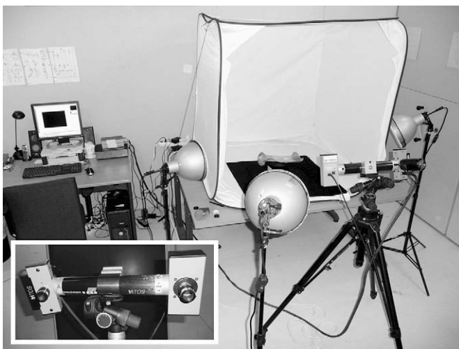
Fig. 1. The Breuckmann triTOS-HE structured light scanner setup in a lab with controlled lighting. The inset shows the front face of the scanner with the projector on the left and the camera on the right. The bone inside the light tent is resting on a turntable controlled by the computer. This scanner communicates with the computer via an external control (the black box sitting next to the computer) (photo by SPM).
