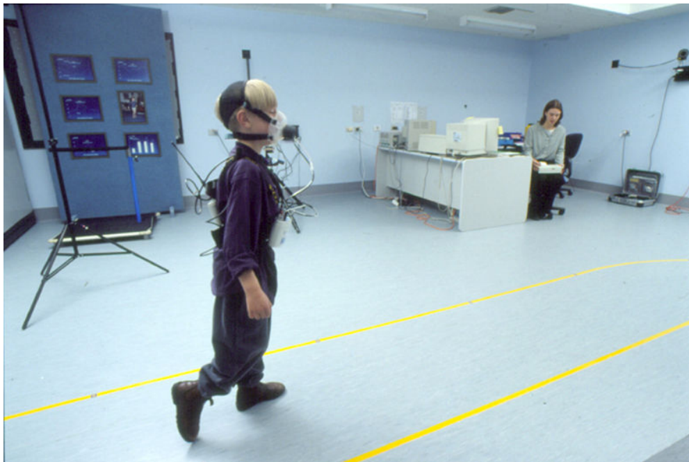
Figure 3.5 A child participating in an energy test in the gait laboratory. The test is conducted on a 20 metre oval walkway (delineated by the yellow lines) within the gait laboratory. The Cosmed K4 unit is an open spirometry system that is lightweight and telemetric. The child is wearing the face mask which directs the expired air to the processing unit which is worn on the front, and the battery pack is worn on the back.
