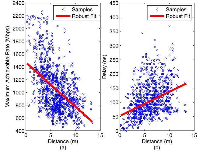
Fig. 5. On the left, maximum achievable rate as a function of distance. On the right, channel delay as a function of distance. In both cases, the linear robust fit is provided.
