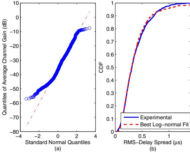
Fig. 2. On the left, quantiles of the average channel gain in dB versus the standard normal quantiles. On the right, cumulative distribution function of the RMS delay spread. The best log-normal fit is also shown.
