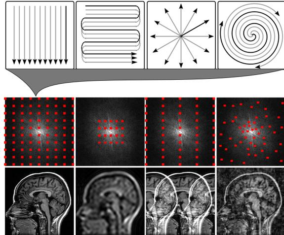
Fig. 2. The Nyquist criterion sets the required  $k$ -space coverage, which can be achieved using various sampling trajectories. Image resolution is determined by the extent of the  $k$ -space coverage. The supported field of view is determined by the sampling density. Violation of the Nyquist criterion causes artifacts in linear reconstructions, which depend on the sampling pattern.
