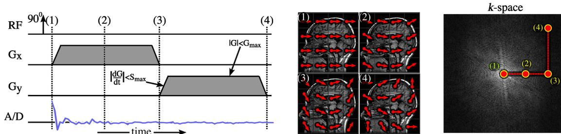
Fig. 1. The temporal MRI signal directly samples the spatial frequency domain of the image. Gradient fields cause a linear frequency distribution across the image, which produces a linear phase accrual with time. The received signals are spatial frequency samples of the image. The corresponding spatial frequencies are proportional to the gradient waveform area. The gradient is limited in amplitude,  $G_{\max}$ , and slew rate,  $S_{\max}$ , which are both system specific.
