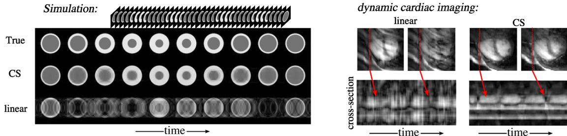
Fig. 11. Dynamic imaging of quasi-periodic change. Left: Phantom experiment showing a reconstruction from 4-fold undersampling. Right: Dynamic acquisition of the heart motion showing a reconstruction from 7-fold undersampling. impossible to meet the spatial-temporal Nyquist rate using this scheme.
