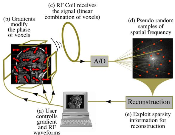
Fig. 4. MRI as a compressed sensing system. The user controls the gradient and RF waveforms which, in turn, control the phase of the pixels/voxels in the image. An RF coil receives the signal in an encoded form – samples in  $k$ -space. Careful crafting of the gradient waveforms allows for incoherent measurements of  $k$ -space. With an appropriate non-linear reconstruction enforcing sparsity, an image can be reconstructed.
