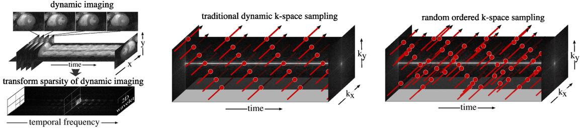
Fig. 7. Left: Dynamic MRI is a multi-dimensional signal with two or three spatial coordinates and time as an additional dimension. Dynamic images have a sparse representation in an appropriate transform domain. Center: Traditional  $k-t$  sequential sampling. Right: Random ordering is an efficient way to incoherently sample the  $k-t$  space.
