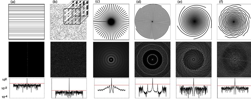
Fig. 6. Point Spread Functions (PSF) of various sampling trajectories. (a) Random lines in 2D (b) Random points in 2D, or cross-section of random lines in 3D (c) Radial (d) Uniform spirals (e) Variable density spirals (f) Variable density perturbed spirals. Height of red lines measures coherence.
