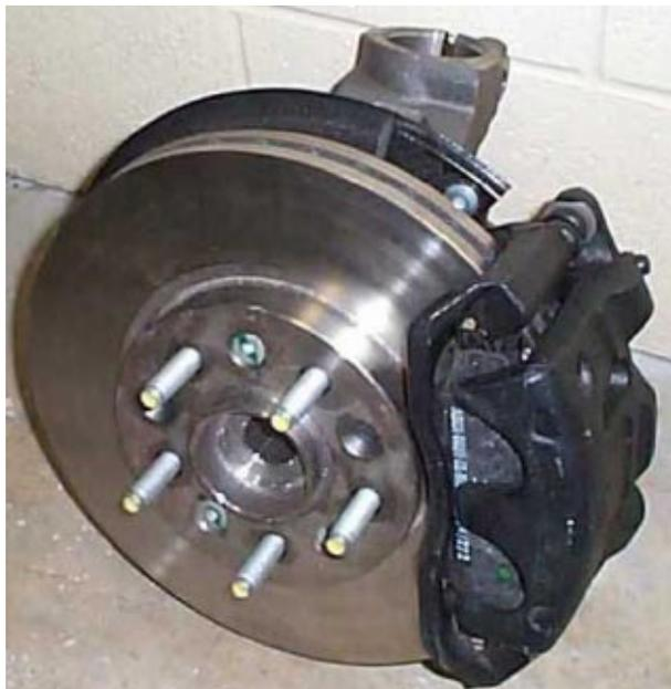
**Fig. 2 Photograph of a typical front wheel automotive assembly excluding the rim and tire**
