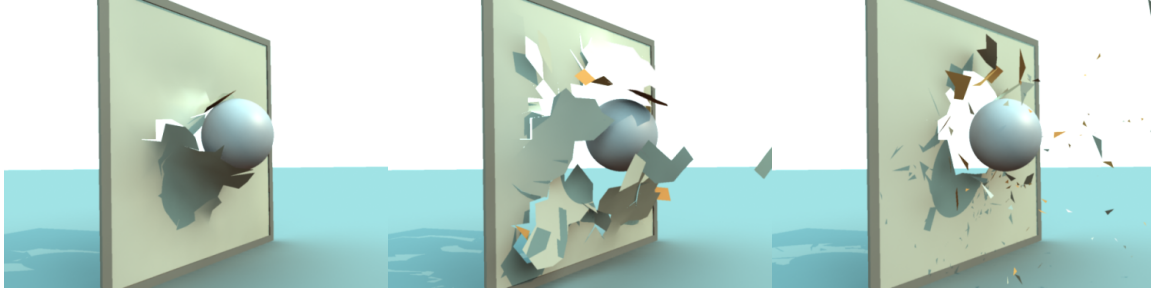
Figure 11: We simulate the puncture of an elastic sheet by a fast projectile. By varying the fracture threshold, \lambda_f , we obtain different behaviors. From left to right, \lambda_f = 0.02, 0.001, 0.0001 .
