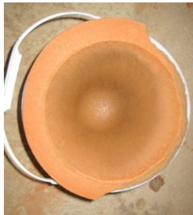
Figure 20. Coffee husk filter (Filter 7) with partially broken rim
