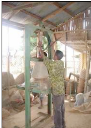
Figure 7. Forming pot shape with a hydraulic press
