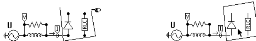
Fig. 3.15 - Drawing a polygon: First double click on white space, click the left mouse button at each corner of the polygon, then click the right button to enclose the polygon.
