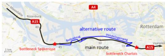
Dependent on the current traffic conditions, BOS-HbR advises to reroute a part of the traffic via the underlying parallel structure. A route-guidance controller is simulated at the bifurcation to the alternative route at Spijkenisse, a second route-guidance controller is simulated after the Botlekbrug. Furthermore, the controllers advice a route for each vehicle class; BOS-HbR distinguishes between cars and trucks.
