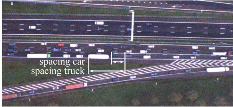
**Figure 2.5: Comparison of spacings of vehicle classes, (frame of a video taken at the Dutch A15R near on-ramp Charlois)**
