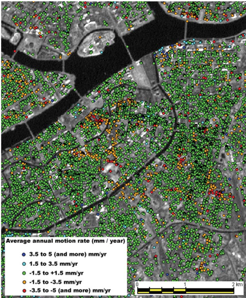
Fig. 3. Map of persistent scatterer points, with their calculated average annual motion rates ( \text{mm year}^{-1} , colour-coded) for St. Petersburg, Russia. PSI data copyright NPA Group 2005; ERS data copyright ESA 1992–2004; background image Landsat ETM + Band 8. (Data processed by NPA for ESA's GMES TerraFirma service.)
