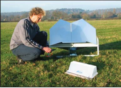
Fig. 5. A metallic Corner Reflector (CR), with a Compact Active Transponder (CAT) in the foreground.
