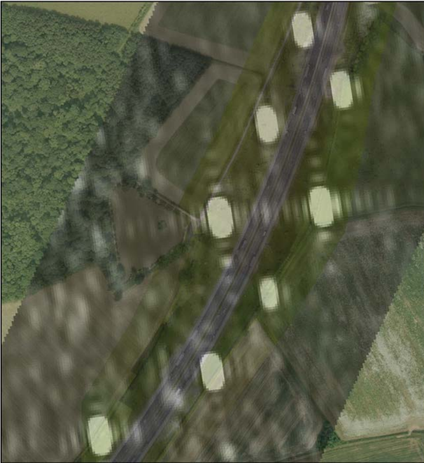
Fig. 6. Intensity responses from a network of NPA's Compact Active Transponders, deployed for monitoring subsidence with InSAR. Image copyright NPA Group 2005.
