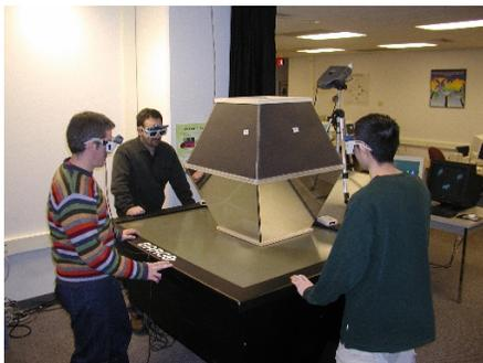
**Figure 2: Our experimental prototype: The Virtual Showcase sits on top of a rear-projection screen. The lower half of the truncated pyramid configuration consists of four half-silvered mirrors. An additional set of full mirrors comprise the top half and redirects the light beam of a video projector (upper right) into the showcase center.**
