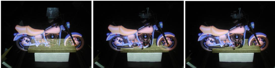
**Figure 3: Knowing the depth information of the real content, also allows the occlusion of virtual objects by real ones (left). Combining this with our occlusion shadow method (center) creates correct mutual occlusion effects between both environments (right).**
