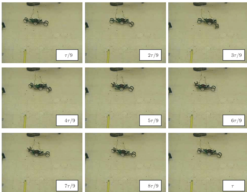
Fig. 15. Several snapshots of the actual kinematic snake while performing a figure-eight type curve. The frames are chosen to depict one complete gait where \tau is the gait's period. Note the small translation of the robot in the x direction. Refer to Extension 2 to watch the original video of this demonstration.
