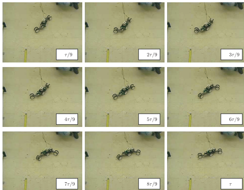
Fig. 17. Several snapshots of the actual kinematic snake while performing a singular figure-eight type curve. The frames are chosen to depict one complete gait where \tau is the gait's period. Note the relatively large rotation of the kinematic snake. Refer to Extension 2 to watch the original video of this demonstration.
