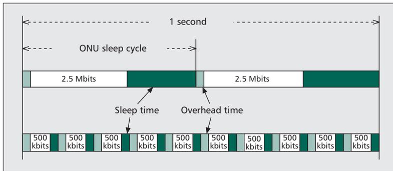
**Figure 4.** Transferring 5 Mb/s traffic using batch-mode (upper diagram) and legacy-mode (lower diagram) transmissions.
