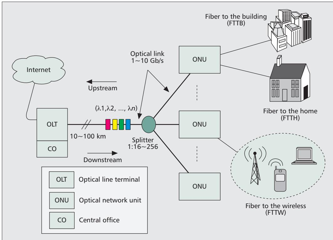
**Figure 1.** Evolution of the NG-PON point-to-multipoint (P2MP) architecture: higher transmission rates, higher split ratios, more ONUs, longer reach, and multiple wavelengths.
