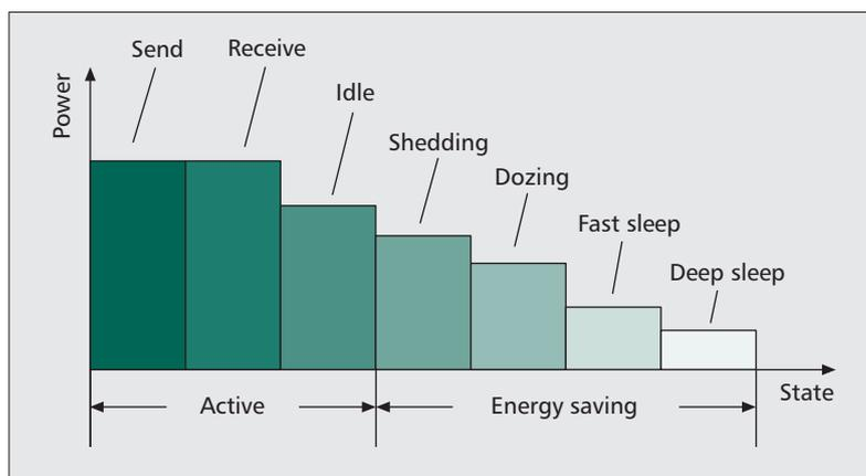
**Figure 3.** ONU power consumption under different active and energy-saving states.
