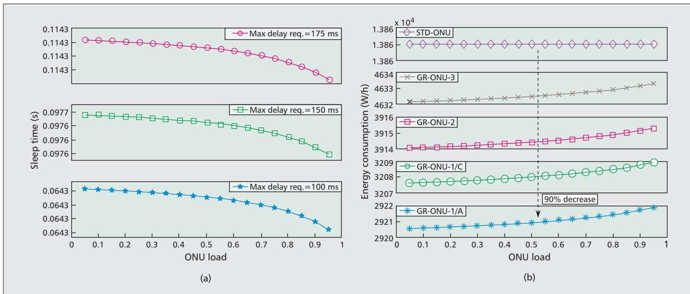
Figure 6. a) Sleep time under GR-ONU-1/A; b) energy consumption of different ONU architectures.
