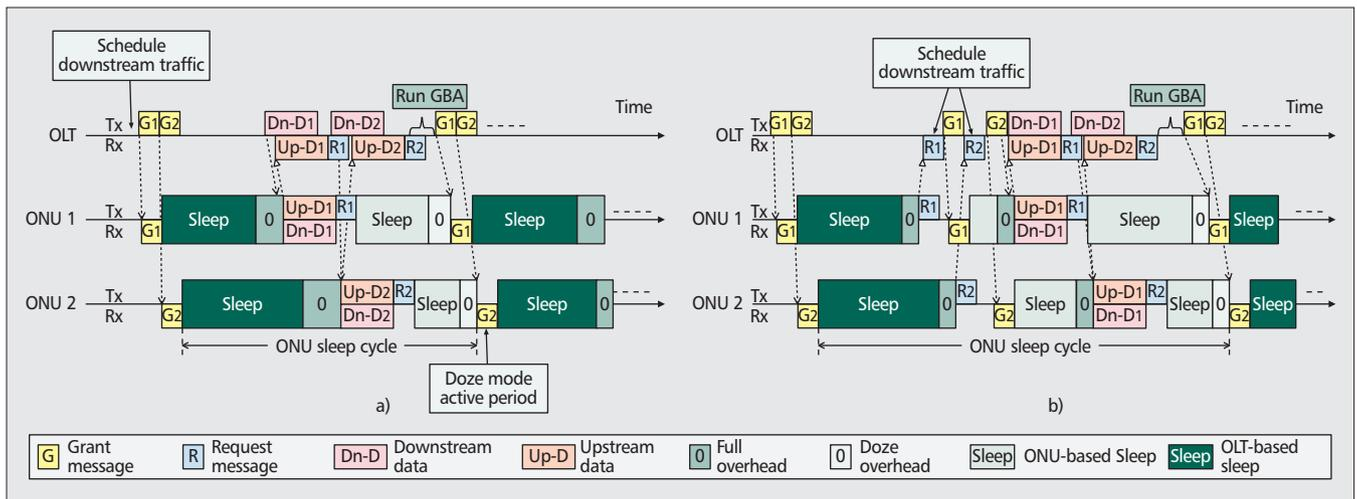
Figure 5. GBA in TDM-based PONs with a) direct ONU transmission; b) request after sleep.
