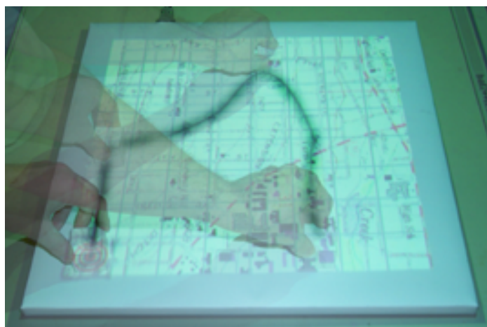
Figure 12: This multiple-exposure photo shows the user tracing out a bus route (enhanced for clarity) using a bus-route-drawing object.
