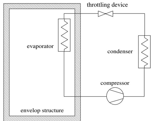
Fig. 1. Basic vapour-compression refrigeration system.
