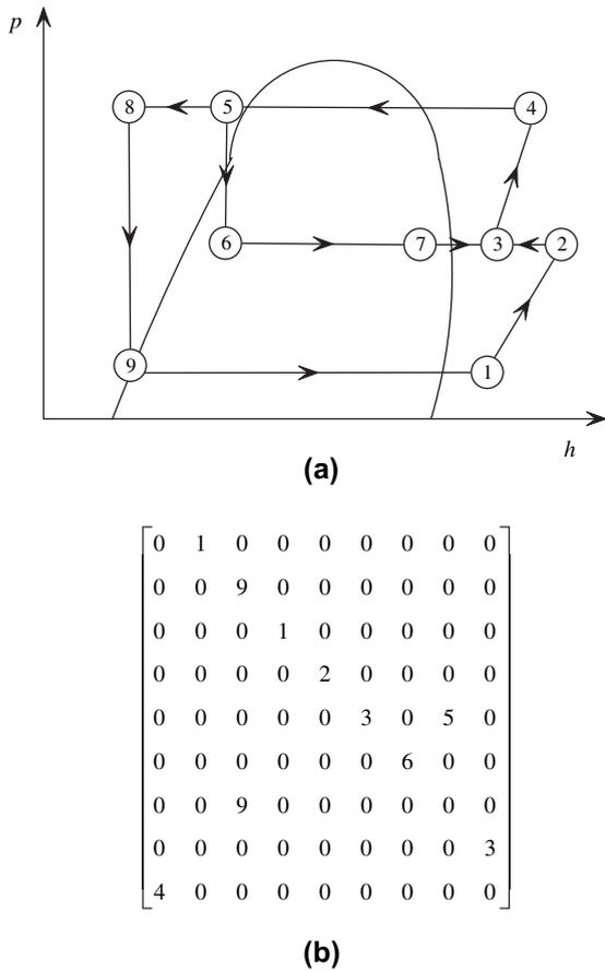
Fig. 5. Graph description for two-stage compression refrigeration cycle: (a) directed graph, (b) matrix.
