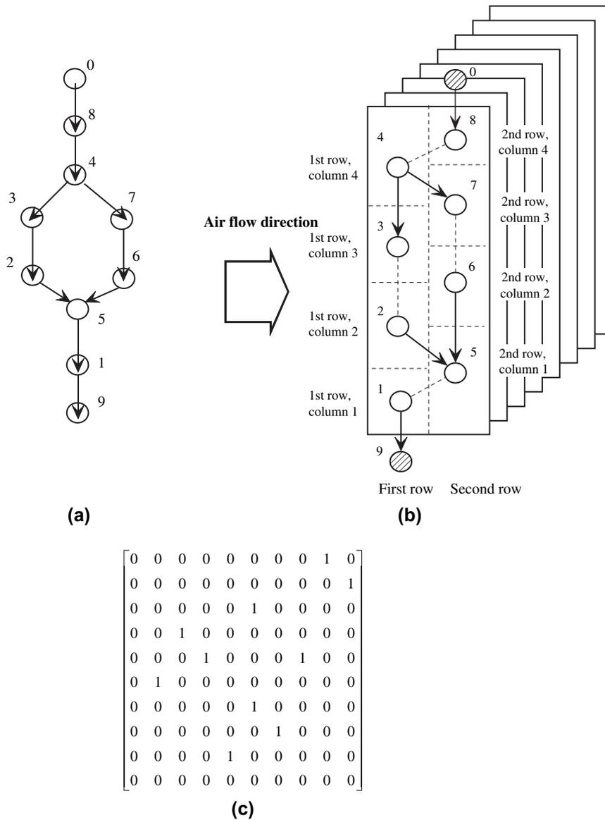
Fig. 6. Graph description for heat exchanger: (a) tube numbering, (b) directed graph, (c) matrix.
