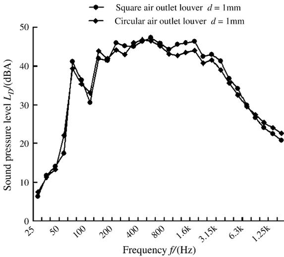
Fig. 7. Influence of shape of air outlet louver on noise generated by the outdoor unit [78].
