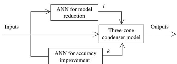
Fig. 3. Schematic of condenser model integrated with ANNs [67].
