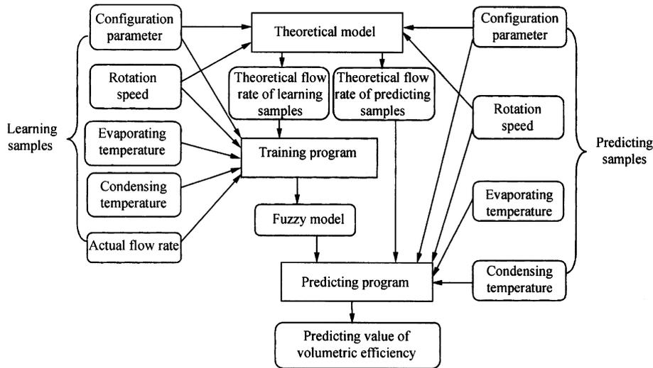
Fig. 4. Fuzzy simulation for volumetric efficiency of refrigeration compressor [68].
