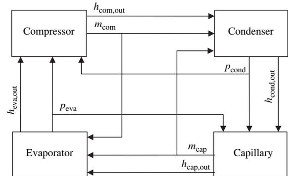
Fig. 2. Coupling of boundary parameters among components.
