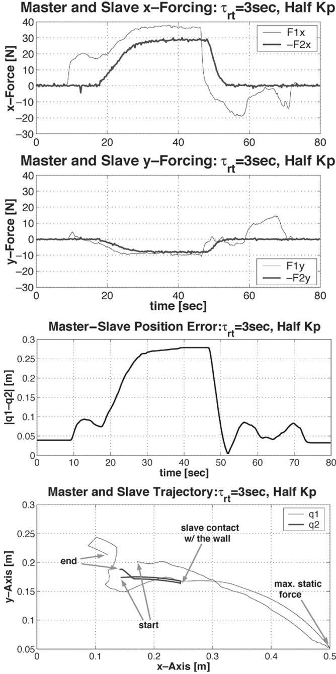
Fig. 8. Experimental results with the round-trip delay  $\tau_{rt} = 3$  s. To enhance motion agility (i.e., to reduce damping force peaks in Fig. 7), the dissipation gain  $K_d$  [also the P-action gain  $K_p$  via (15)] is reduced by half.
