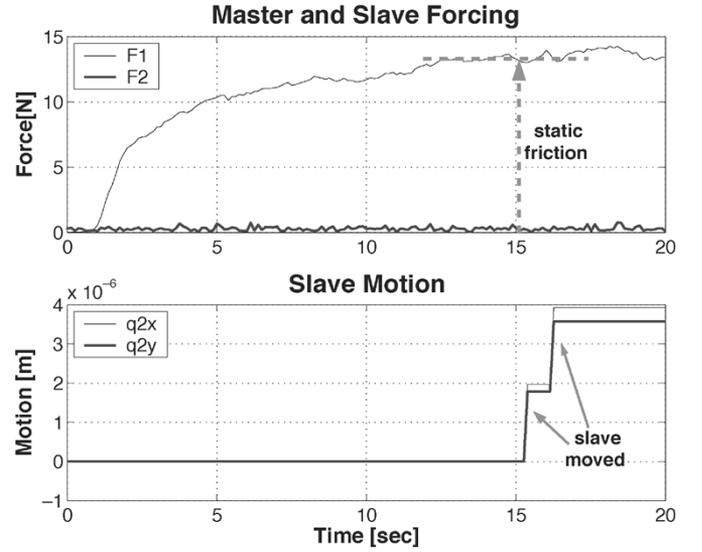
Fig. 5. Coulomb friction in the experiment system.
