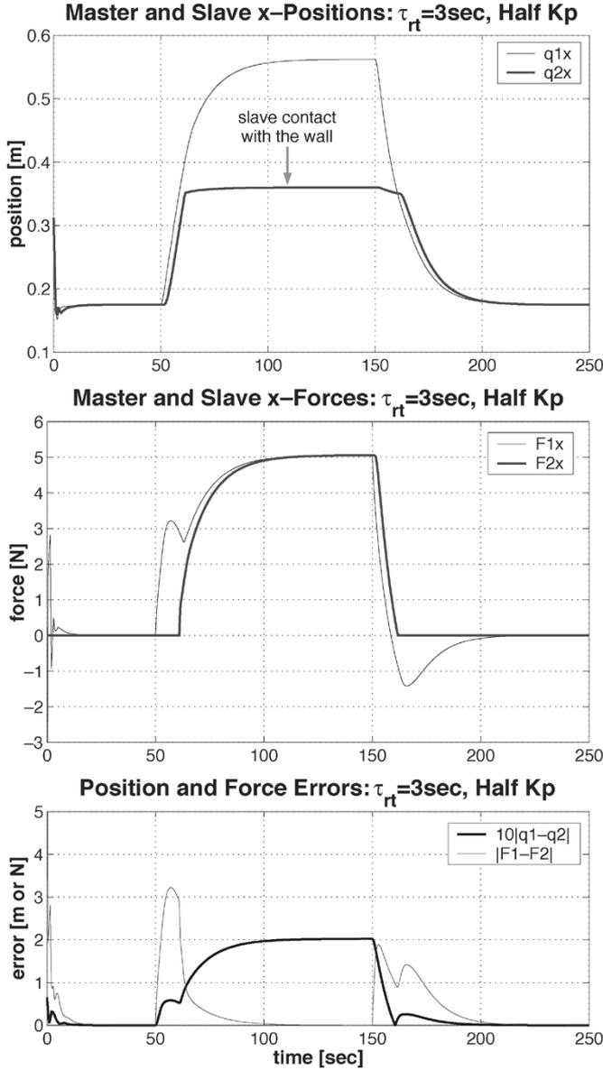
Fig. 4. Simulation result:  $\tau_{rt} = 3$  s,  $K_p = 25I_{2 \times 2}$ ,  $K_d = 37.5I_{2 \times 2}$ . To enhance motion agility (i.e., reduce the damping force peaks in Fig. 3), the dissipation gain  $K_d$  [also, the P-control gain  $K_p$  via (15)] is reduced by half from Fig. 3.
