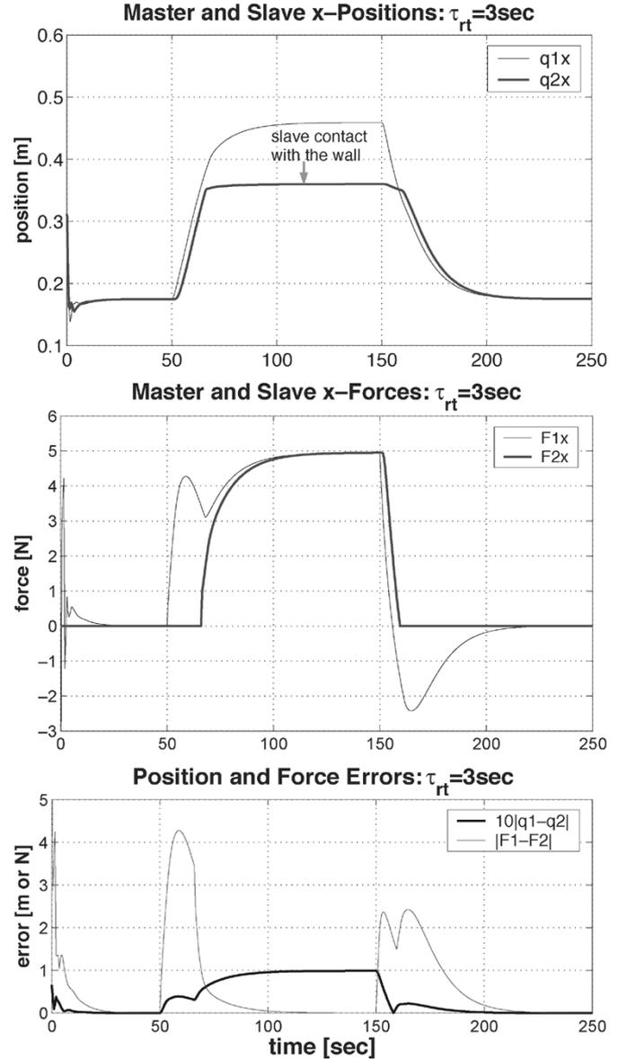
Fig. 3. Simulation result:  $\tau_{rt} = 3$  s,  $K_p = 50I_{2 \times 2}$ ,  $K_d = 75I_{2 \times 2}$ .
