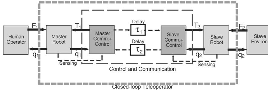
Fig. 1. Closed-loop teleoperator as a two-port system, where the dotted arrows represent information flow through the delayed communication channels, while solid arrows represent mechanical power pairs.
