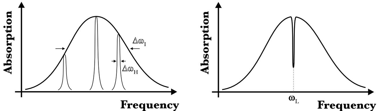
Figure 7: (a) Inhomogeneously-broadened absorption spectrum. (b) After illumination with a narrowband laser at  $\omega_L$ , a persistent spectral hole has been “burned” into the absorption spectrum. (After Reference (245)).
