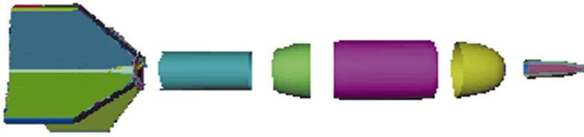
Fig. 17. Several subassemblies of the dart model isolated via region extraction.
