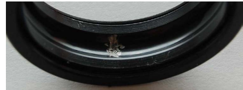
FIGURE 3. Bearing with a large outer race defect
