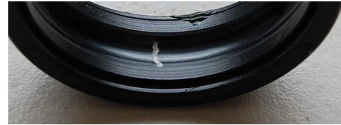
FIGURE 2. Bearing with a small outer race defect
