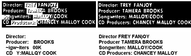
Figure 4. Thresholding (using BAT method, which is to be presented later) and recognition results after averaging on all text-frames (left column) and HCFs (right column) (Character/word recognition rate: left – 0.483/0.357, right – 0.966/0.857).
