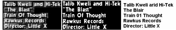
(c) Results of HCB averaging, BAT thresholding and recognition. Totally there are 68 characters/14 words. Our algorithm can correctly recognize 65 characters/12 words, while without HCF/HCB averaging and BAT we can only correctly recognize 50 characters/7 words.
