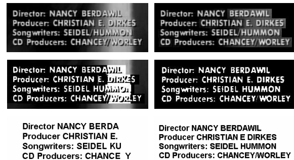
Figure 7. Comparison of HCF averaging and HCB averaging. The left column are averaging, thresholding (using BAT method, which is to be presented later) and recognition results using HCF averaging, while the right column is the corresponding results using HCB averaging (Character/word recognition rate: left – 0.783/0.643, right – 1.0/1.0).
