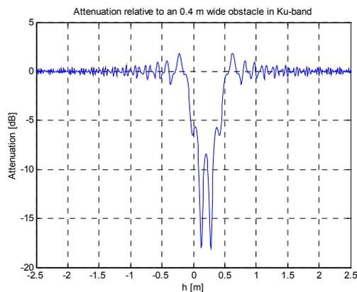
**Figure 3. Attenuation Due to an Electrical Bridge**
