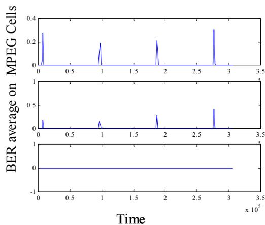
**Figure 9. Average BER with and without Block Channel Int..  $v = 120$  km/h,  $SNR > SNR_{QEF}$**
