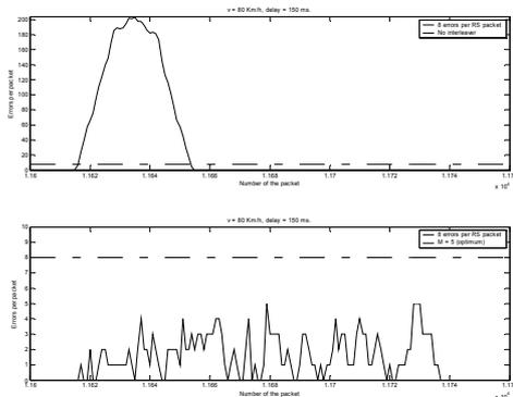
Figure 6. Numbers of Errors per Packet When Crossing an Electrical Bridge
