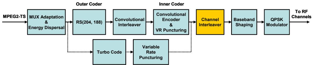
Figure 5. Modified DVB-S/DVB-RCS Based Air-Interface for the FIFTH System
