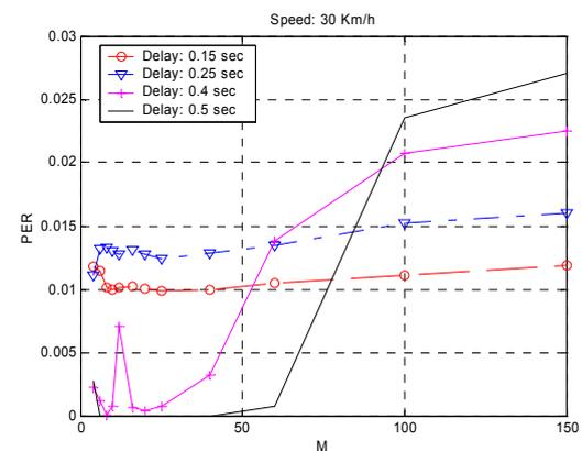
Figure 8. PER for Different Delays and Low Train Speed
