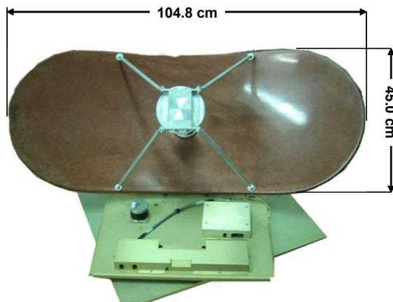
**Figure 4. The FIFTH Terminal Antenna**
