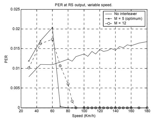
Figure 7. PER for Different Convolutional Interleavers
