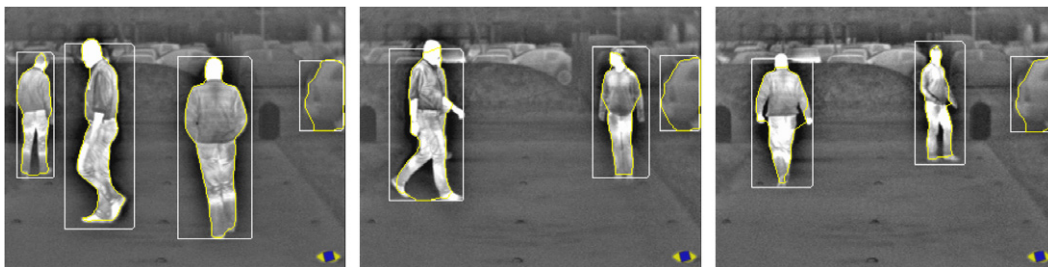
Fig. 11. Shape detection results: the white rectangles are the bounding boxes where the snakes are initialized and the yellow curves represent the final positions of the snakes.
