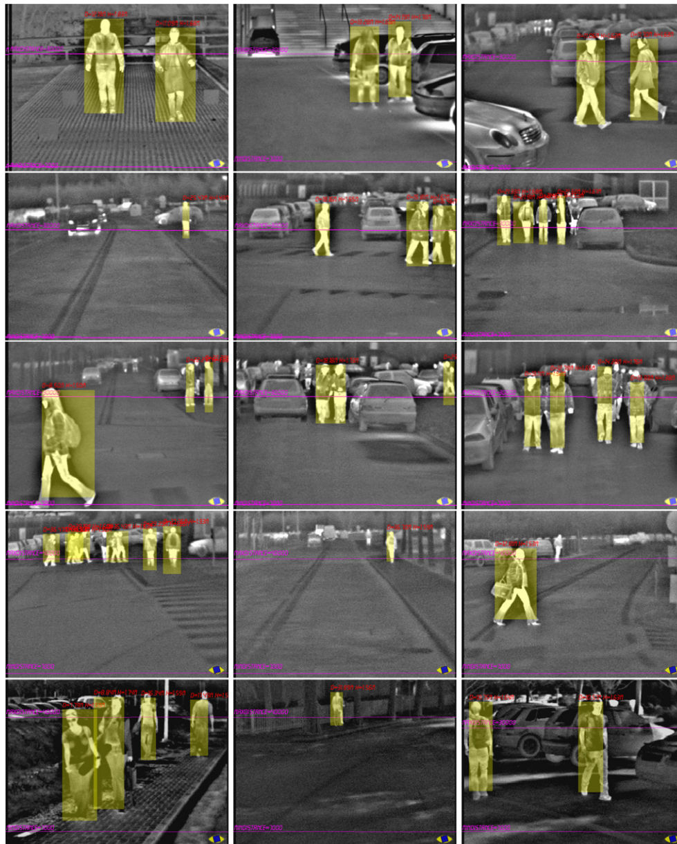
Fig. 8. Pedestrian detection results: detected pedestrians are shown using a superimposed yellow box. Each box also shows the distance and height of detected object. The two magenta lines show the minimum and maximum distances used for the detection.
