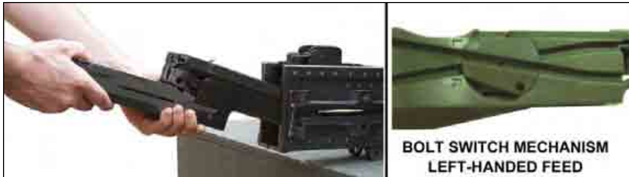
* Figure 2-18. Returning the barrel extension, barrel buffer, and bolt groups together.
