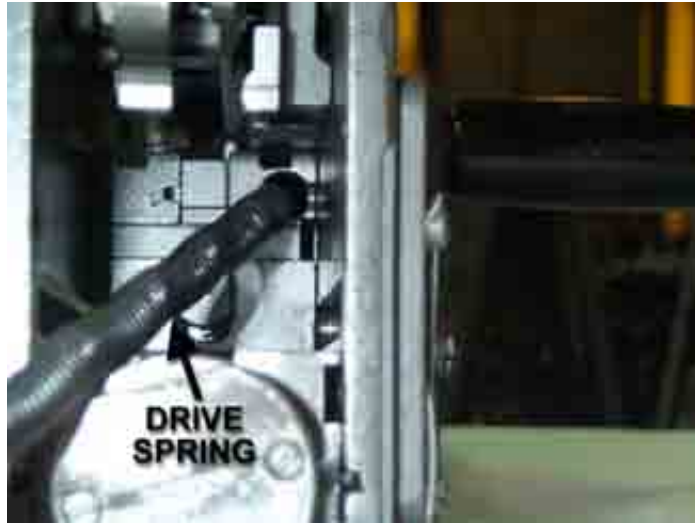
* Figure 2-20. Inserting drive spring and drive spring rod (with drive spring rod inside drive spring).
