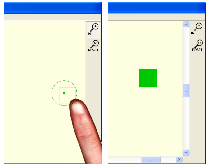
Figure 1. Zoom-Pointing: First the user zooms to a sub-area defined by drawing a rectangle (left). The user can then perform direct pointing at a finer scale (right). The figure shows a square target, highlighted by a surrounding circle.
