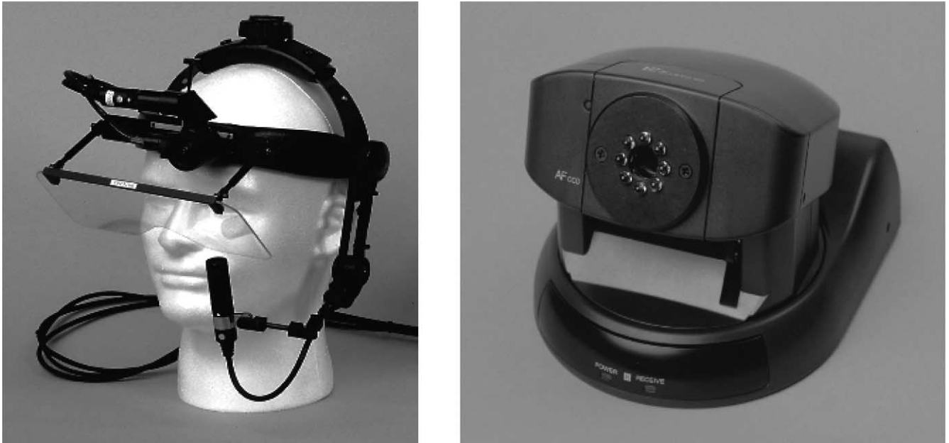
Fig. 7. Examples of eye trackers manufactured by Applied Science Laboratories (ASL): (a) model ASL-501 (accuracy 0.5–1.0°, visual range 50° (H), and 40° (V), sampling rate 50–60 Hz with optional increase to 120–240 Hz) and (b) ASL-504 with remote optics (accuracy 0.5°, visual range 50° (H), and 40° (V), sampling rate 50–60 Hz with optional increase to 240 Hz). Image courtesy of Applied Science Laboratories.
