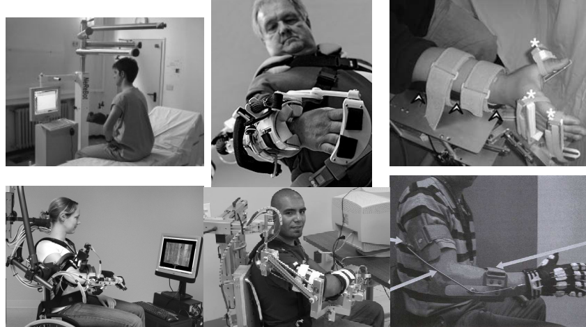
Figure 4. Recently developed robotic and non-robotic therapy devices. Upper left: NeReBot: a 5 DOF cable robot that can be used next to a patient's bed [27]. Bottom left: ArmIn: a highly responsive robot that allows naturalistic arm movement, including shoulder translation [28]. Middle top: Rupert: a lightweight exoskeleton actuated with pneumatic muscles, which can be worn by the subject [29]. Middle bottom: T-WREX – a non-robotic arm support device [21]. Upper right: HWARD – a 3 DOF hand and wrist robot [23]. Lower right: A cable driven glove that can be worn, and driven by a motor or the patients shoulder shrugs [30].
