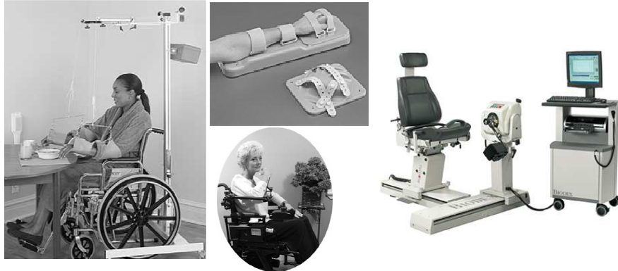
Figure 1. Pre-cursors of robotic therapy devices. The three devices on the left (Swedish sling, arm skateboard, and JAECO mobile arm support) are designed to provide assistance for arm movement without using actuators. The device on the right is the Biodex Active Dynamometer, which is a single degree-of-freedom robot that can be adjusted to assist or resist movement around different joints.
