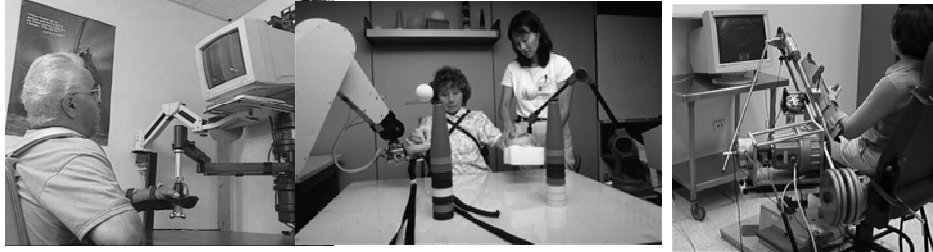
Figure 2. Some of the first robotic therapy devices for the arm to undergo clinical testing (left to right: MIT-MANUS [2], MIME [4], the ARM Guide [5]). These devices were designed to provide active assistance to patients during reaching movements with the arm.
